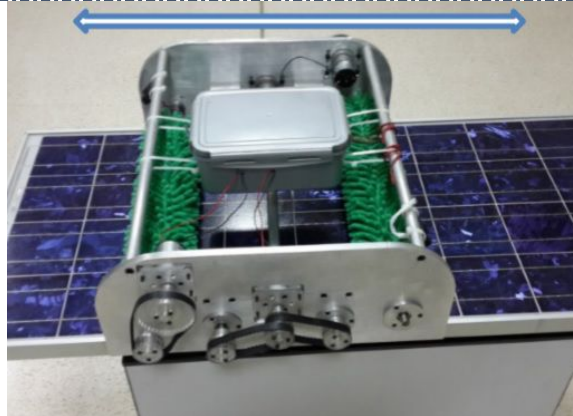
Fig. 6 Direction of cleaning system.
